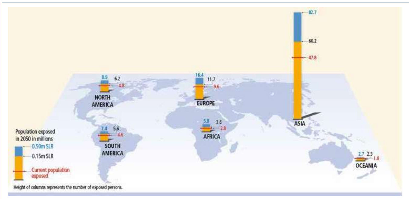
Figure 1. For low-elevation coastal areas, current and future (2050) population exposure to inundation in the case of the 1-in-100-year extreme storm for a sea-level rise of 0.15 m and for a sea-level rise of 0.50 m due to the partial melting of the Greenland and West Antarctic Ice Sheets (Handmer et al., 2012; data from Lenton et al., 2009)
